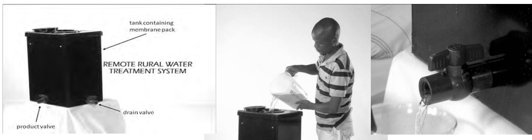
Figure 3: Rural Water Treatment Unit and Its Operation
