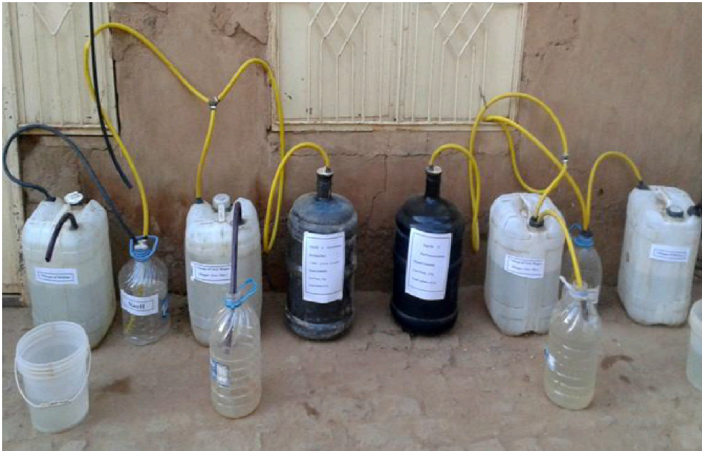
Figure 4: Bio-digesters (D1) and (D2) installed in experiment system
