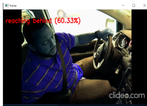
Figure 4: System classifying that the driver is reaching for something at the back of the car
