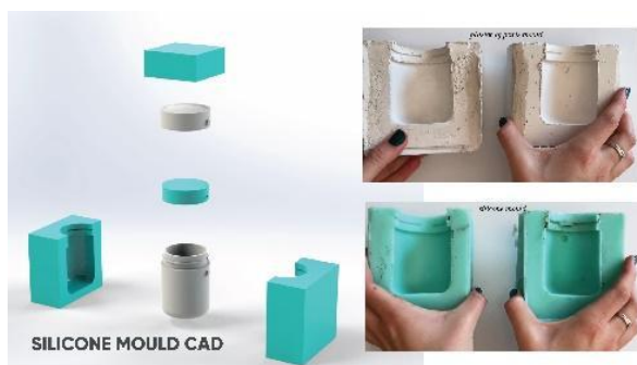
Figure 8: Low-tech tooling, utilized for biomaterial production
