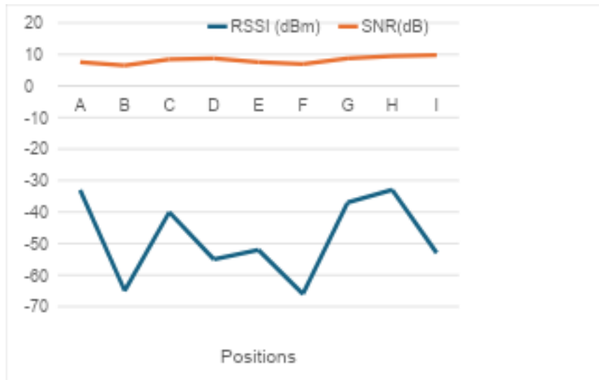
Figure 6: The LoRaWAN coverage measurements and results
